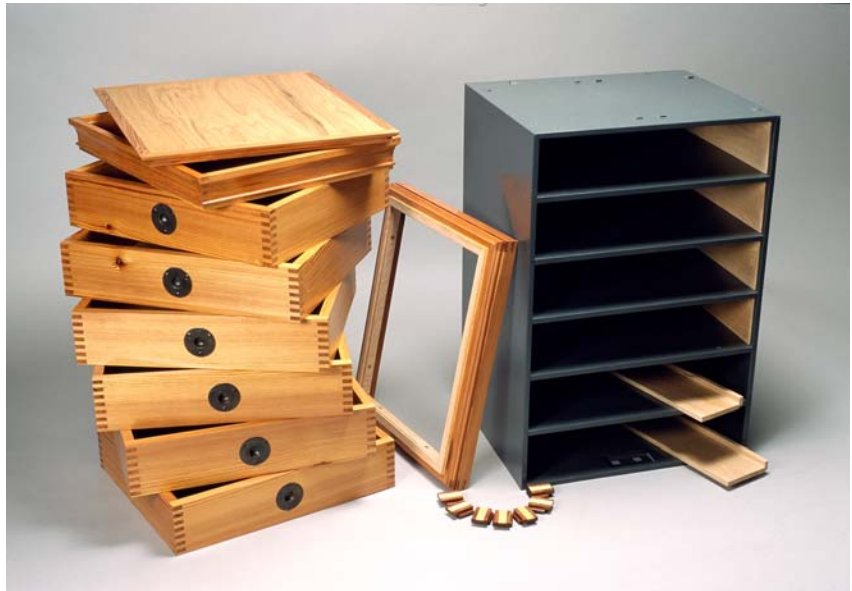
Picture 4: The Case of Drawers’ components: Crown molding or Box, drawers, base, drawer stops (cleats) and glides as well as the original filing cabinet.
